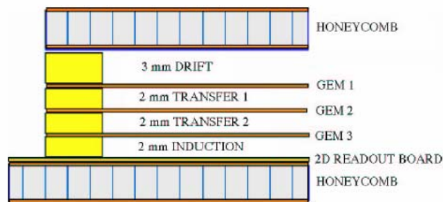
Fig. 5. The spacing between the various components in the triple GEM.
